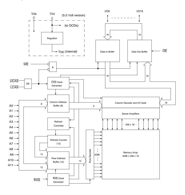
IBM0116160 IBM0116160M IBM0116160B IBM0116160P **1M x 16 12/8 DRAM**
